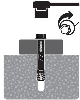
With correct size socket or spanner tighten anchor to specified torque. Installation complete!
