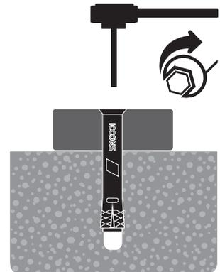
With correct size PH3 driver bit tighten anchor to specified torque. Installation complete!
