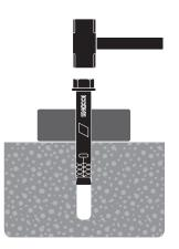
Insert anchor into position.
