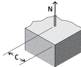
To achieve published tension loads the anchors should be installed at least 8 x the anchor drill diameter from a concrete edge. If edge distance is closer than 8 x the anchor drill diameter apply the appropriate reduction factor as outlined in the EDGE DISTANCE TENSION TABLE to the published load to ascertain the reduced load.
