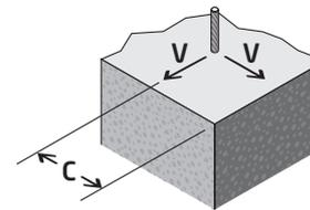
To achieve published shear loads the anchors should be installed at least 12 x the anchor drill diameter from a concrete edge. If edge distance is closer than 12 x the anchor drill diameter apply the appropriate reduction factor as outlined in the EDGE DISTANCE SHEAR TABLE to the published load to ascertain the reduced load.
