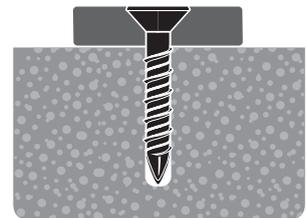
Continue to tighten the anchor until countersunk head is firmly seated against fixture. Installation complete!
