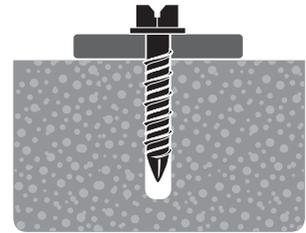
Continue to tighten the anchor until hex head is firmly seated against fixture. Installation complete!
